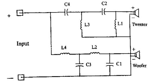
$$C_1 = \frac{.1040}{R_{RH}(F \times 1.13)} \times 1,000,000 \quad L_1 = \frac{.1009 \times R_{RH}}{F \times 1.13} \times 1,000$$
