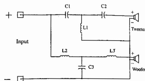
$$C_1 = \frac{.1061}{R_H \times F} \times 1,000,000 \quad L_1 = \frac{.1194 \times R_H}{F} \times 1,000$$
