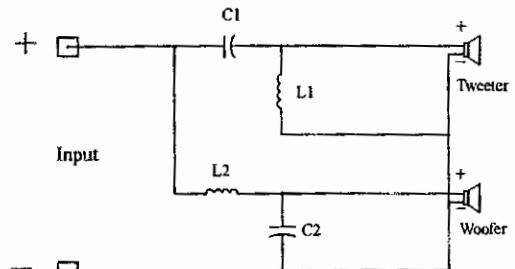
$$C_1 = \frac{.1125}{R(F \times 1.3)} \times 1,000,000 \quad L_1 = \frac{.2251 \times R}{(F \times 1.3)} \times 1,000$$
