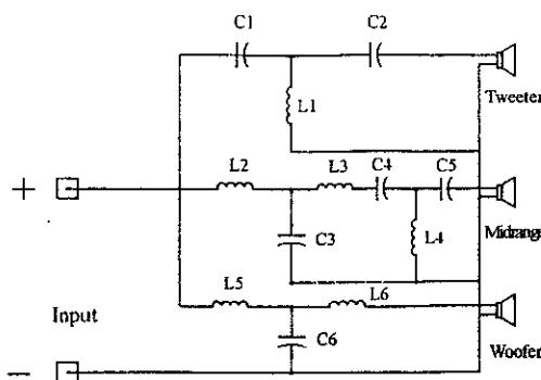
$$C_1 = \frac{.1158}{R_{RH} \times F_H} \times 1,000,000 \quad L_1 = \frac{.1189 \times R}{F_H} \times 1,000$$
