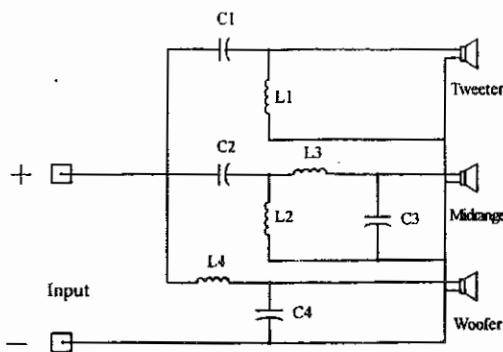
$$C_1 = \frac{.0791}{R_H \times F_H} \times 1,000,000 \quad L_1 = \frac{.3202 \times R_H}{F_H} \times 1,000$$
