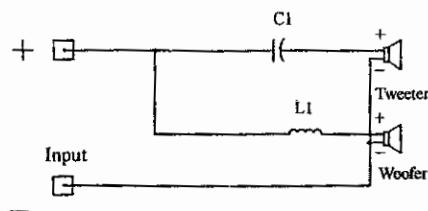
$$C_1 = \text{Capacitor} \quad X_C = \frac{1}{2\pi F_c R} \times 1,000,000$$
