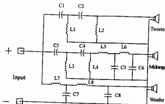
$$C_1 = \frac{0.0848}{R_H \times F_H} \times 1,000,000 \quad L_1 = \frac{1.004 \times R_H}{F_H} \times 1,000$$
